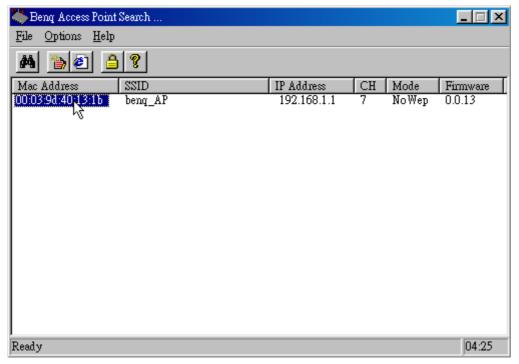
III. When the Access Point is found within the network, a configuration window will appear. You will see the basic information of the Access Point, such as MAC Address SSID IP Channel WEP Mode and Firmware Version.
